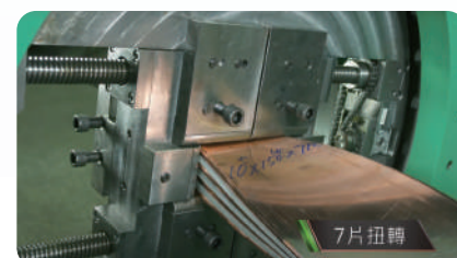
Torsion : 10t*150w*7pcs busbar
